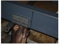
b) The base has to be drilled in the two holes of the bottom of the U-profile with a 5 mm Ø drill.
