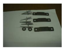
a) For fixation of the visible part of metal strip on the rear panel will be three metal brackets  $80 \times 20 \times 1,5$  mm (20732) installed. The top bracket must be fixed approximate 80 mm below the end of the pipe. The other two should follow at a distance of approximately 545 mm. 5 mm holes must be drilled in the rear panel before riveting with the six blind rivets  $4.8 \times 17$  mm (19968).
